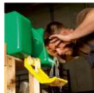
Portable Eye Wash Station
