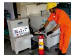
Refilling & HPT of Fire Extinguishers
